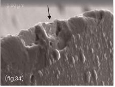
Microscopic photo of chipping and wear marks on the cutting edge of a milling cutter.
