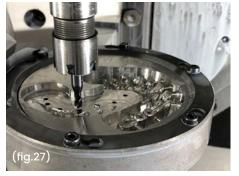
A toric milling cutter in the process of roughing the workpiece, slowly appearing to "emerge" from the raw material.
