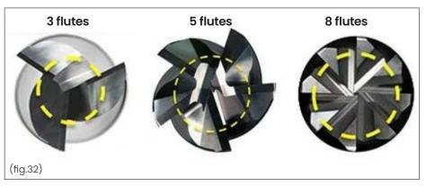
From left to right, a front view of milling cutters with 3, 5, or 8 flutes. There are milling cutters with as few as a single flute and increasing from there. Note that as the number of flutes increases, the diameter of the cutter's central core also increases, while the chip space of each flute decreases.
