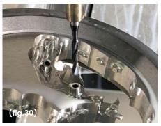
A drill bit used in an intermittent drilling operation. Note the precisely calibrated hole created in the raw material.
