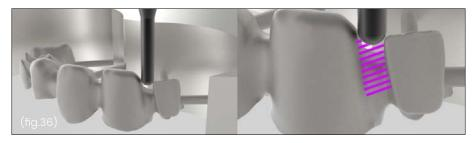
If the working part of the milling cutter has too large a diameter, it will be impossible for the cutter to access the entire surface of the file to be reproduced. As a result, certain areas of the file may not be reproduced at all unless 5-axis toolpaths or smaller cutters are used. In this example, the inaccessible area for a hypothetical spherical cutter with a Ø2mm diameter is marked.
