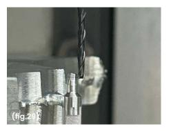
A cylindrical milling cutter.
