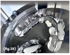
A spherical milling cutter engaged in a finishing or copy milling operation, where the cutter moves along the surface of the workpiece, grazing it tangentially.
